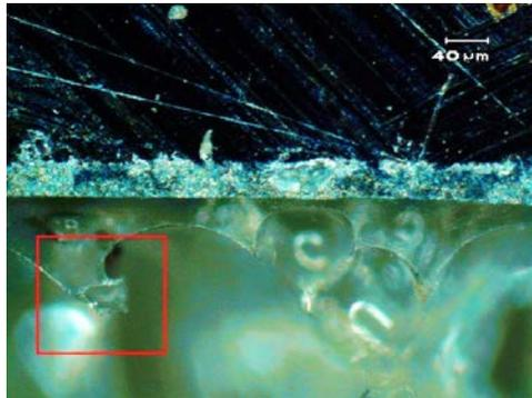
**Figure 4. A typical optical microscope image of the foam-metal interface (using Dark field and 100× total magnification) showing steel (black), zinc (silver), and polyurethane foam**
