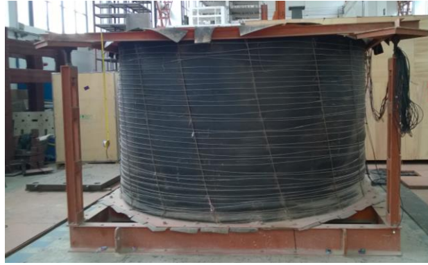
Figure 1. Shaking table and soil container
