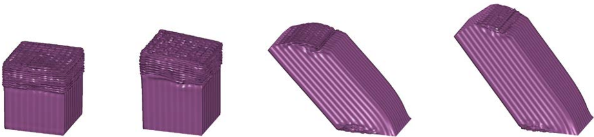
Fig. 4 Deformation modes of multi-cell tubes with different cell number N
