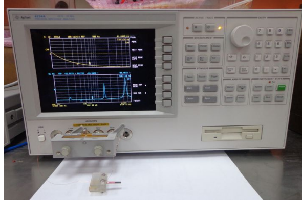
Fig.6 Test system for sensor sensitivity measurement
