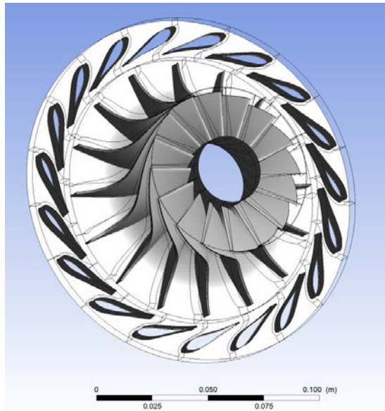
Figure 1. Rotor and Stator geometry of the radial-inflow turbine
