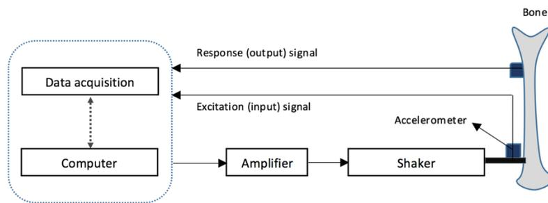
**Figure 2. Measuring vibration response of bone using shaker**
