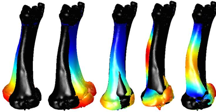
**Figure 6. The first five natural modes of vibration; clamped-free BCs**
