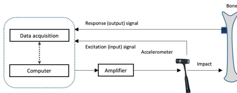
**Figure 3. Measuring vibration response of bone using modal hammer**
