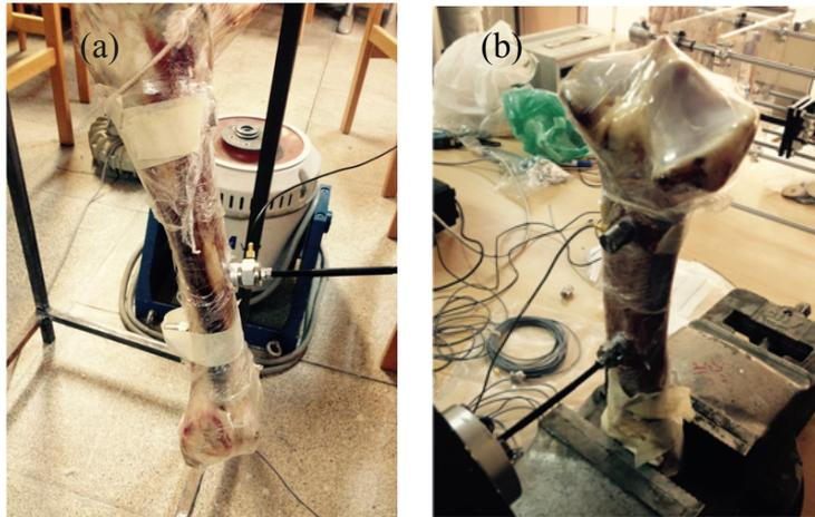
**Figure 1. Shaker test setup; (a) free-free (b) clamped-free BCs**
