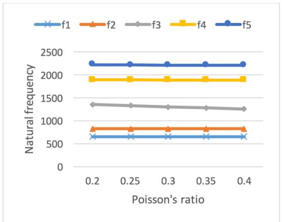
**Figure 10 sensitivity analysis Poisson's ratio**
