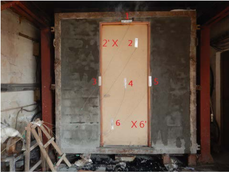
Figure 2. Single leaf - door installed on the furnace
