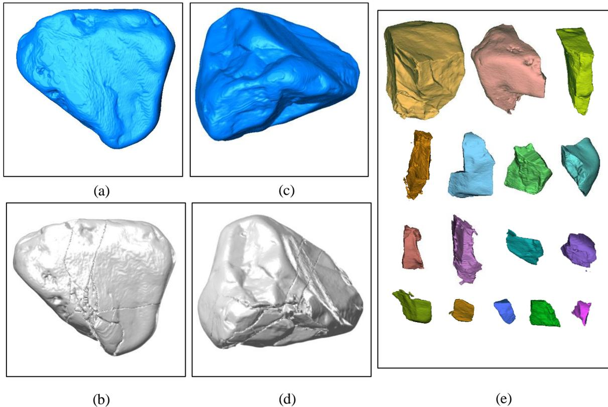
**Fig. 1. LBS-1 model: (a, c) the original particle shape; (b, d) the reassembly result; (e) 3D fragment model**
