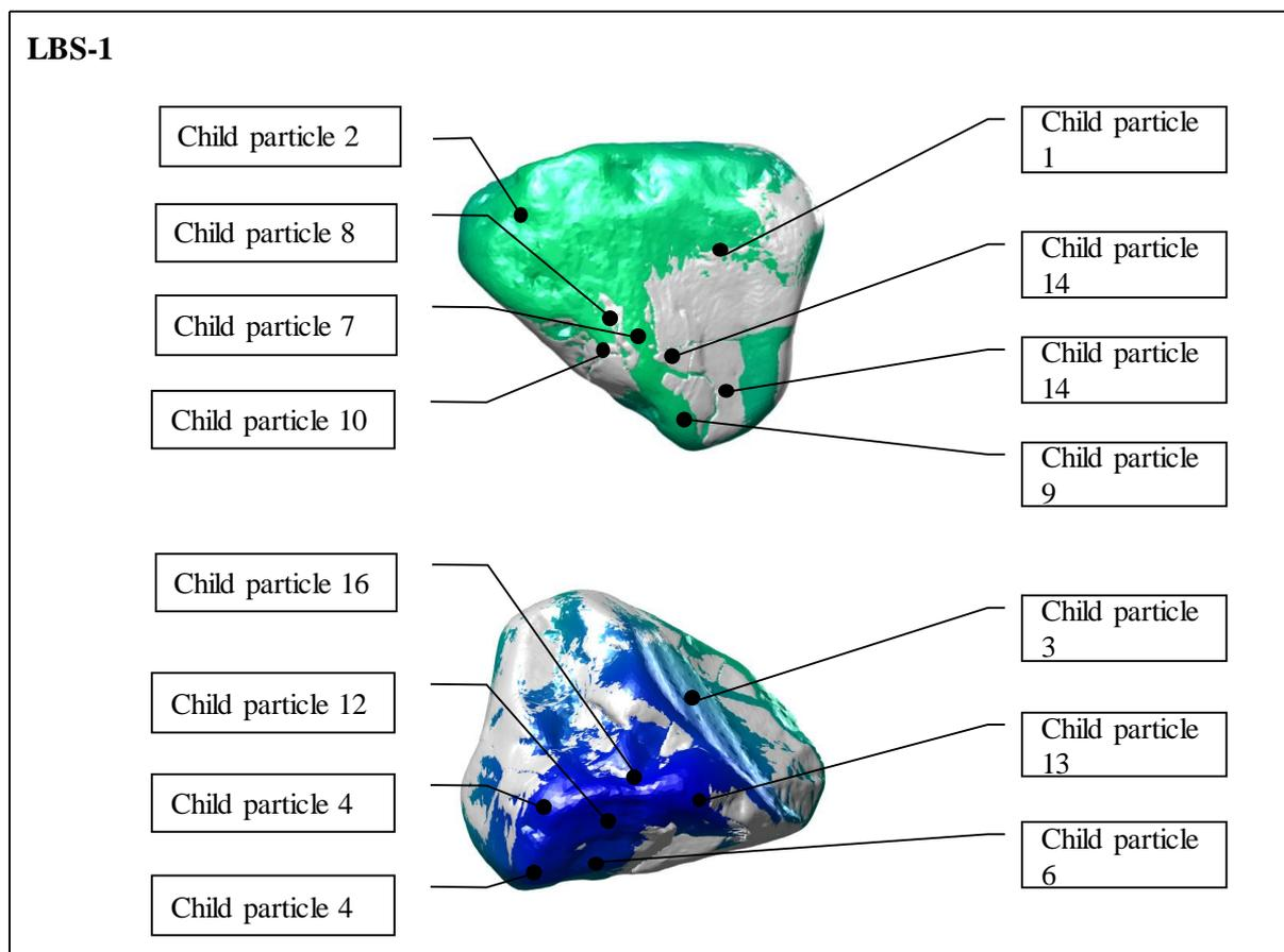
**Fig. 3. Group A: the original and fracture face information for a given child particle (The grey color expresses the child particle and the mother particle is presented by the rest color.)**
