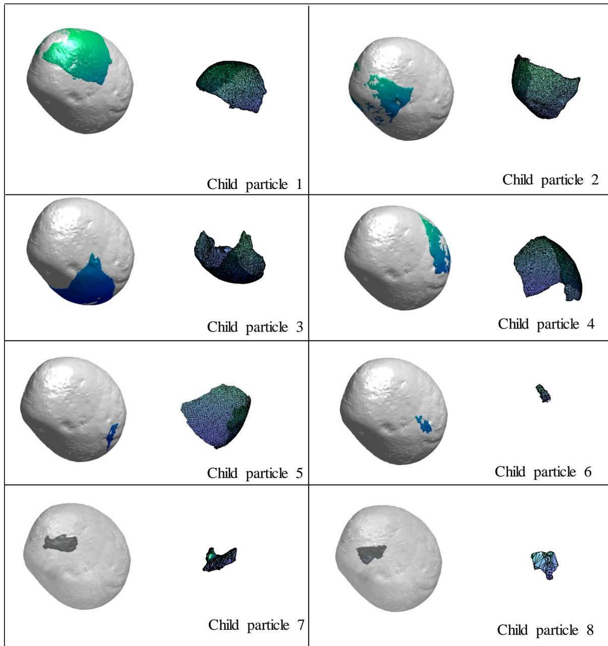
**Fig. 4. The results of image matching between child particle and mother particle (The grey color expresses the mother particle and the child particle is presented with green color. The mesh expresses the region with higher point density. Translucent state exists in the child particle 7 and 8 for better observing.)**
