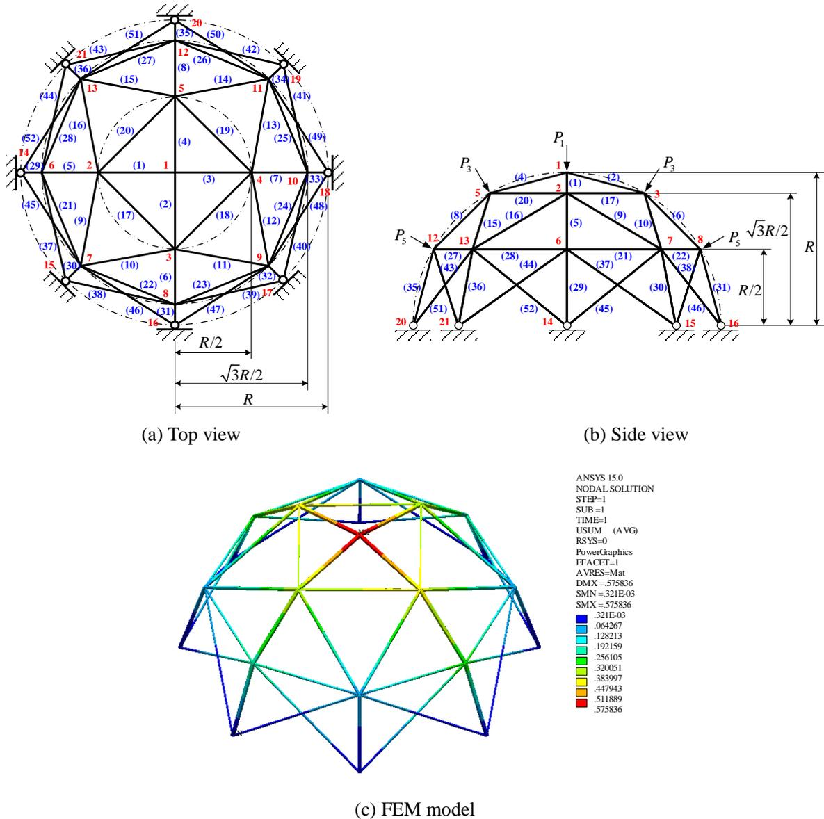
**Fig. 1.** The 52-bar space truss and its FEM model
