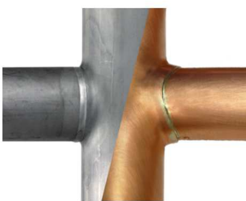
Fig. 1.The example of traditional (left) and formed by flanging T-pipe joint (right) [1]
