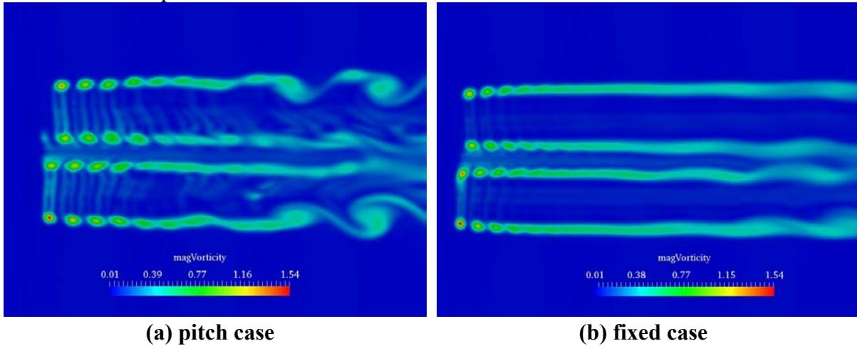
**Fig. 12 Visualization of instantaneous ( $t=170s$ ) vorticity counter at horizontal plane with the height of hub center ( $z=90m$ ).**
