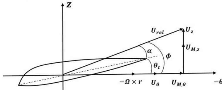
**Fig. 1 Velocity at cross-sectional airfoil element**
