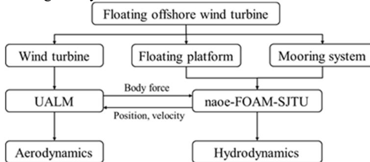
**Fig. 2 Schematic diagram of the coupled analysis tool**
