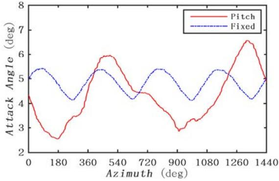
**Fig. 8 Comparison of the attack angle at  $r/R=0.8$  of the rotating blade.**
