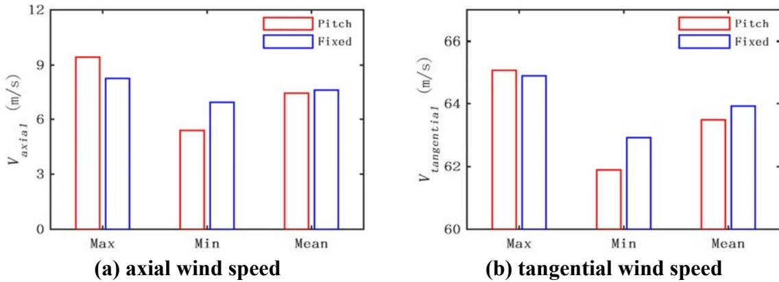
**Fig. 7 Characteristic values of relative wind speed experiencing by blade #1 at a typical blade cross section  $r/R=0.8$  during the rotation of wind turbine.**
