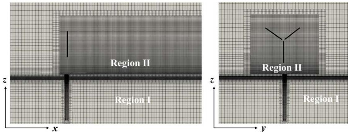
**Fig. 5 Grid distribution in longitudinal section and cross section**
