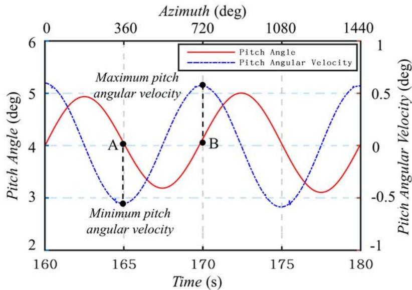
**Fig. 6 Pitch responses of the floating support platform under operating wind and wave conditions.**
