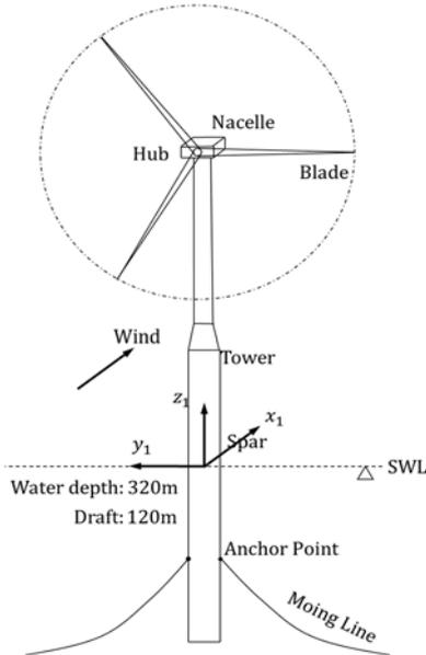
**Fig.3 Diagram of the FOWT system**
