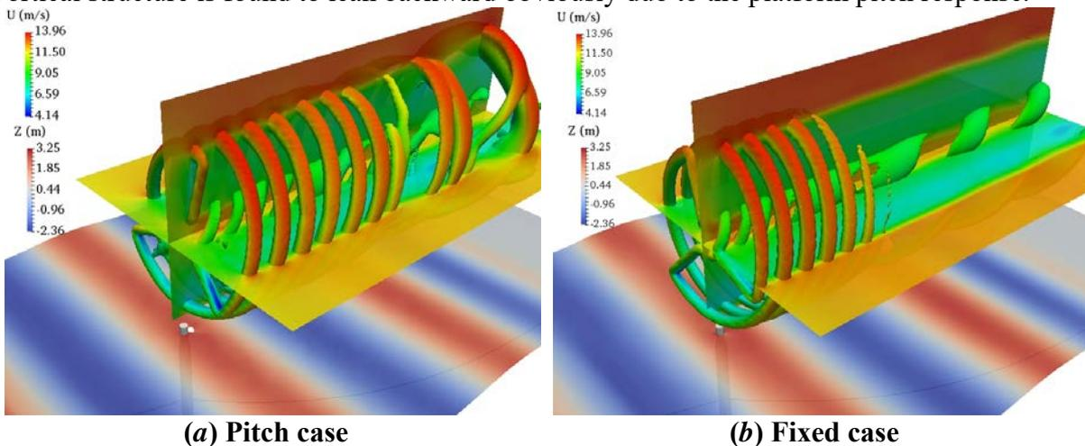
**Fig. 13 Illustration of coupled simulations for the FOWT where the wake vortex is counted by  $Q=0.01$  and colored by wind speed.**
