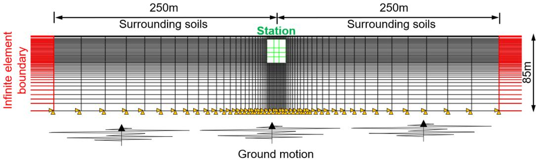
**Figure 2. Numerical model of the underground subway station with surrounding soils**
