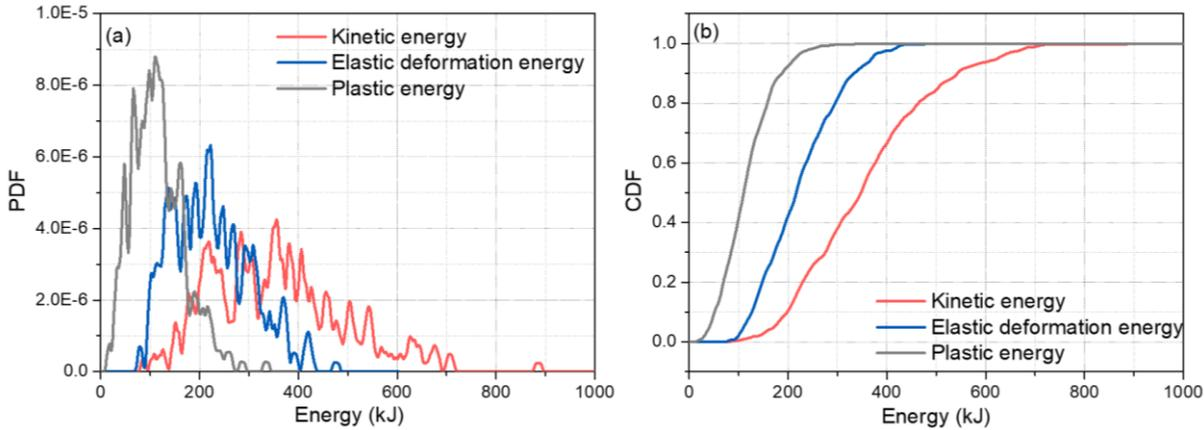
**Figure 7. PDF and CDF curves of maximum energy during earthquake**
