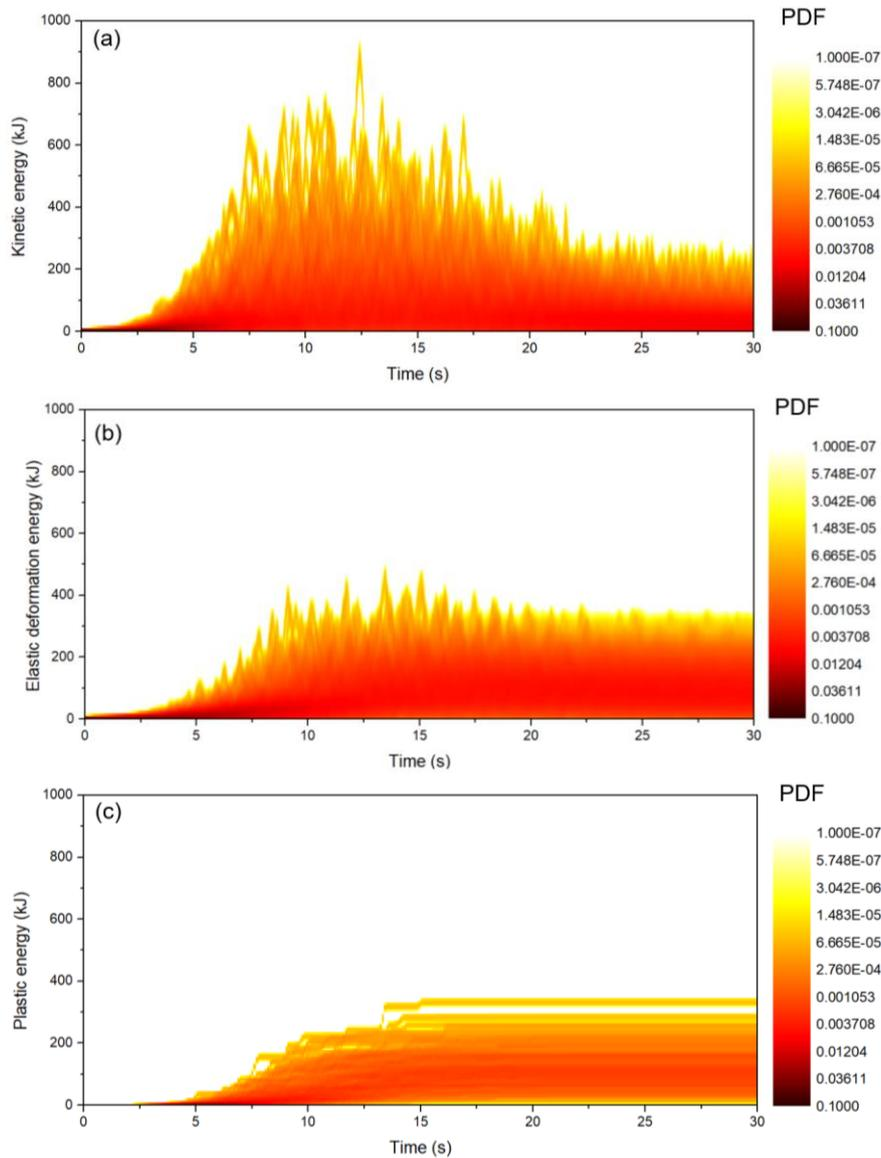
**Figure 5. PDF evolution contours of (a) kinetic energy; (b) elastic deformation energy and (c) plastic energy dissipation of the structure**
