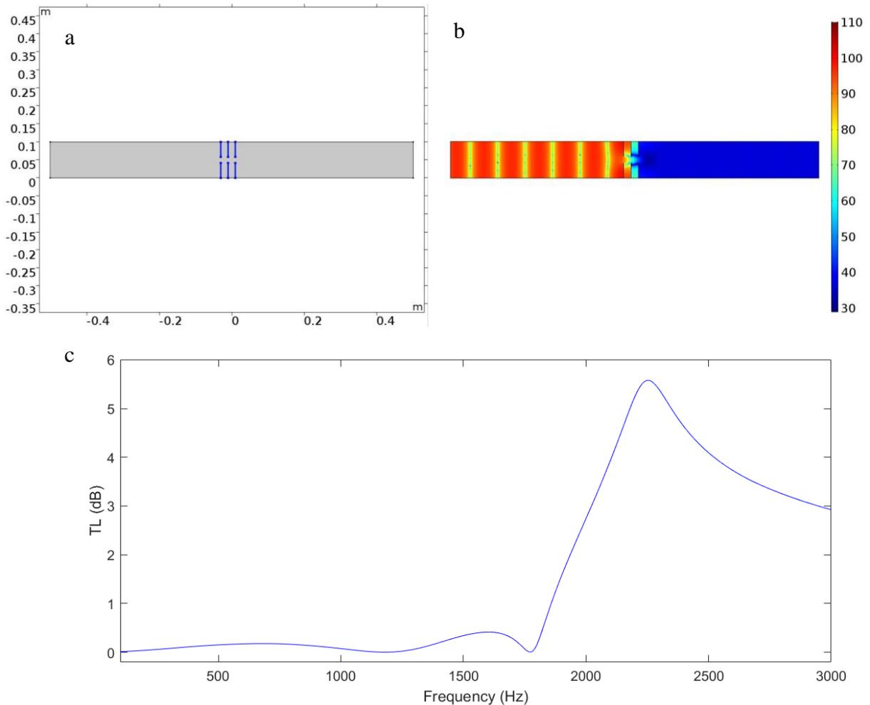
Figure 8. TL Parametrisation for straight duct reproducing the one in Design 2: (a) geometrical setting (internal boundary conditions in blue), (b) SPL distribution at peak frequency 2300 Hz, (c) TL.
