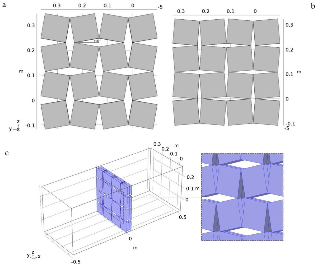
Figure 2. Geometrical configurations of Design 2, frontal view of  $10^\circ$  configuration (a) and  $5^\circ$  configuration (b). Schematic of interior sound hard boundaries, highlighted in blue (c).
