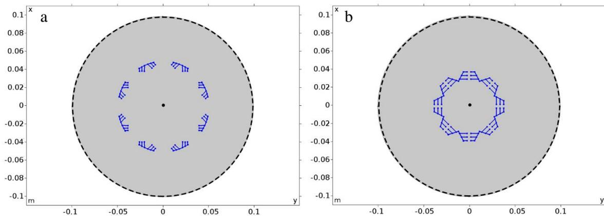
Figure 1. Geometrical configurations of Design 1 unfolded (a) and folded (b) and boundary conditions: central point source, interior sound hard boundaries (blue), and cylindrical free wave radiation (dashed line).
