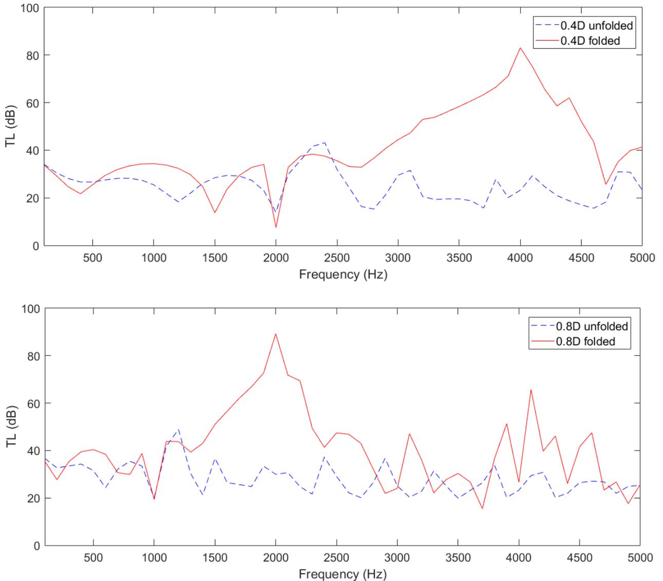
Figure 6. TL comparison of Design 1 (unfolded and folded) with different diameters dimensions (0.2, 0.4, and 0.8 m).
