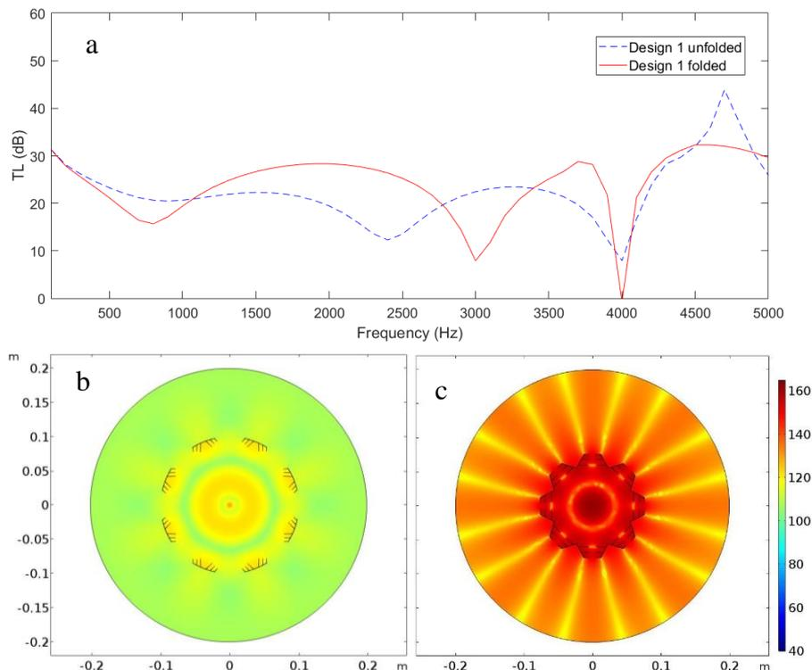
Figure 4. TL (a) and SPL distribution graph for 0.2 m Design 1 at 3000 Hz of the unfolded (b) and 3900 Hz of the folded configuration (c).
