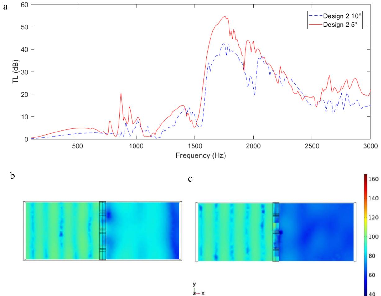
Figure 7. TL (a) and SPL distribution graph for Design 2 10° at 1800 Hz (b) and Design 2 5° at 1700 (c).
