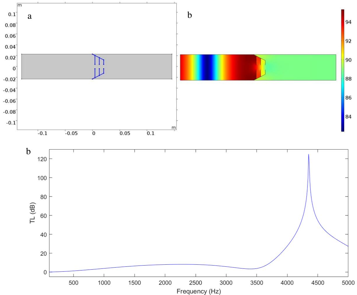
Figure 5. TL Parametrisation for conical duct as the one in Design 1: (a) geometrical setting (internal boundary in blue), (b) SPL distribution at peak frequency 4400 Hz, (c) TL.
