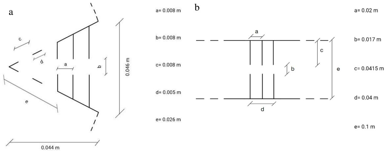
Figure 3. Schematic and dimensions of the metamaterial unit formed in the folded state for Design 1 (a), and of Design 2 (b).
