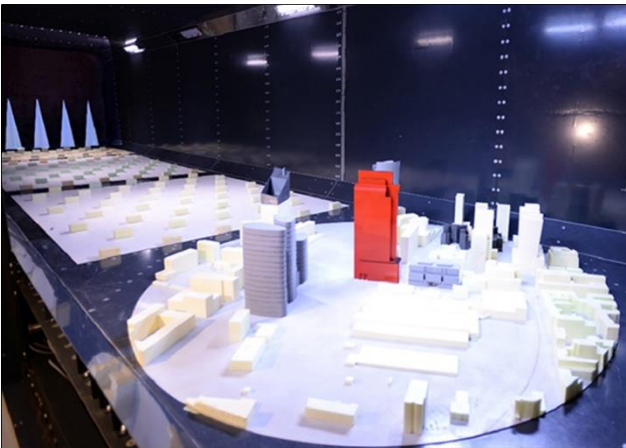
Figure 5. Model of the analysed building and the surrounding in the wind tunnel
