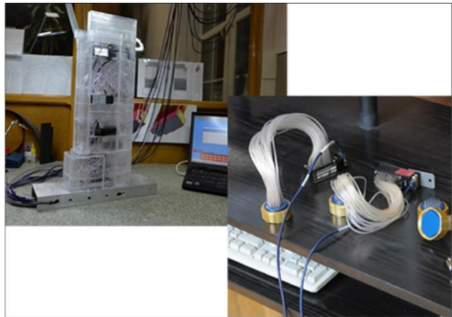
Figure 6. Pressure sensors – installed inside the model and connected to quick-release couplings
