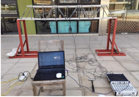
Figure 12 Experimental model of steel frame bridge.
