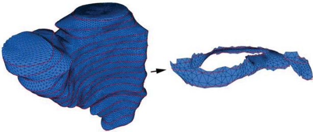
Figure 2. A Sub-mesh is a subset of the 3D mesh that is bounded by a pair of contour lines.
