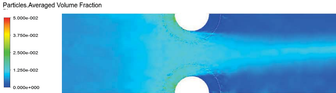
Figure 7: Averaged Volume Fraction of Particles for the steady simulation at U_{\infty}=3 m/s
