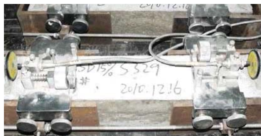
Fig 3 Non-contact concrete shrinkage test
