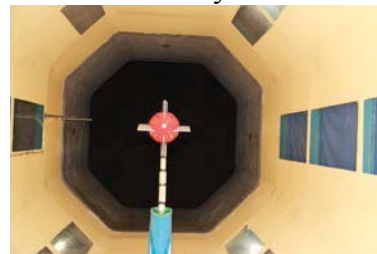
Figure 6. Elevators deflection angle change test
