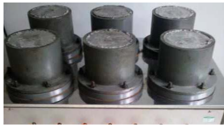
Fig 1 Concrete permeability automatic recording instrument
