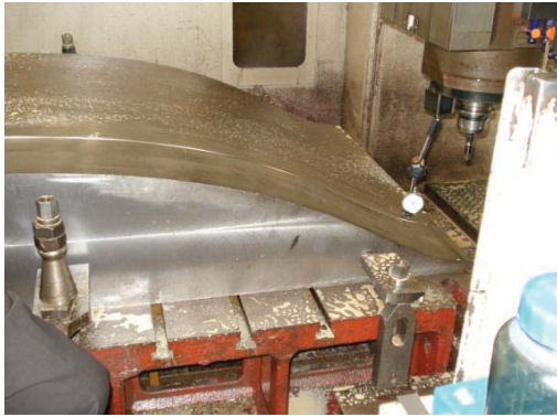
Figure 15. Using alloy steel welded for M3.5 nozzle
