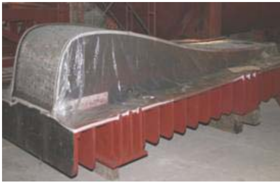
Figure 1. The frame foundation of epoxy resin surface
