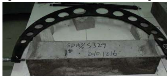
Fig 4 Contact concrete shrinkage test
