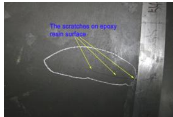
Figure 4. The scratches on epoxy resin surface
