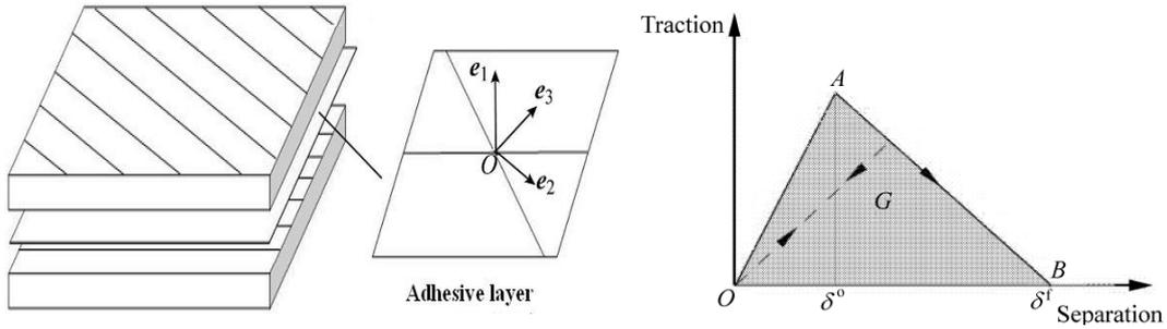
Fig.1 Mechanics model of the laminates Fig.2 Interface force-relative displacement
