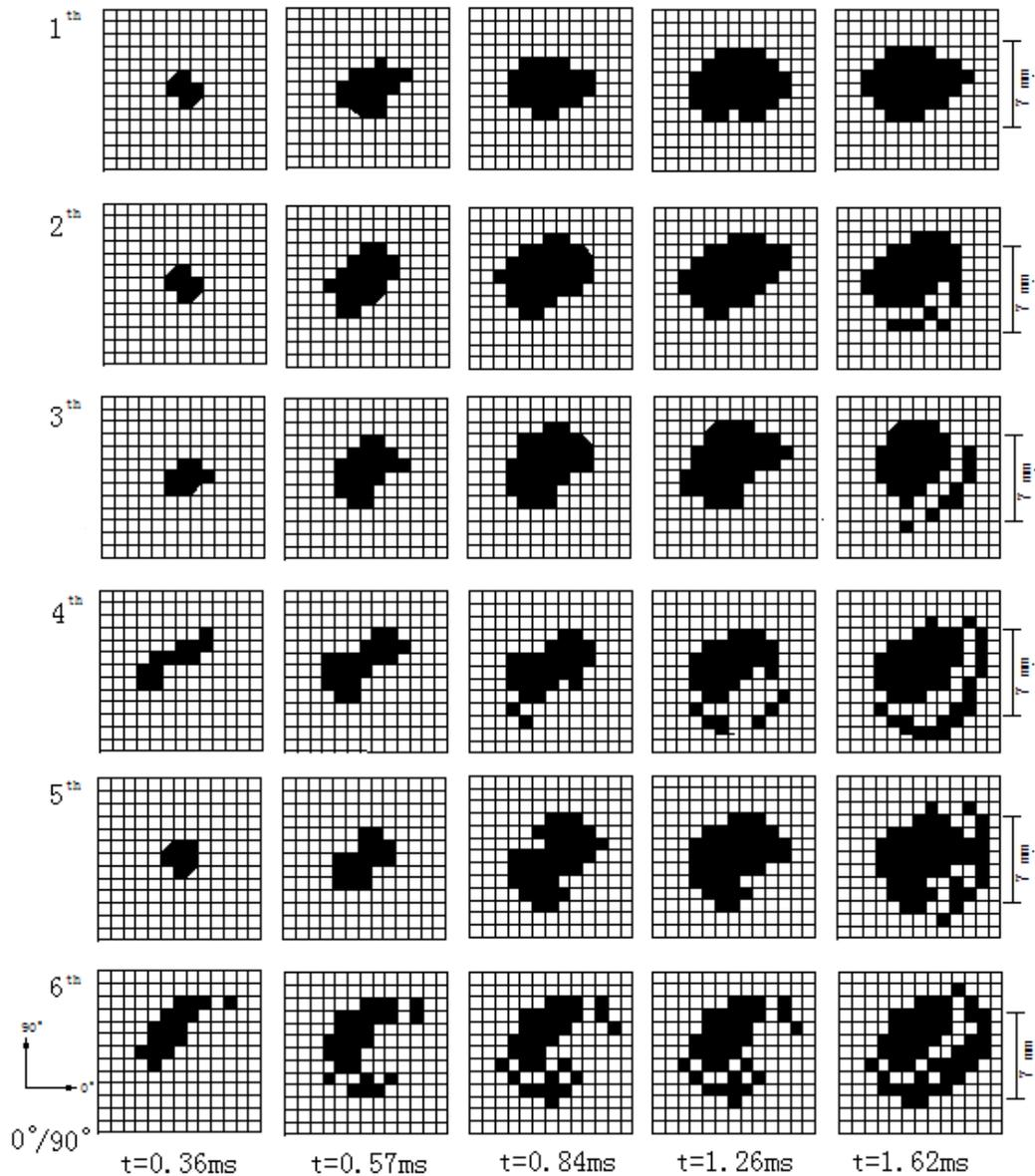
**Fig.6** Delamination damage growth images in adhere layers
