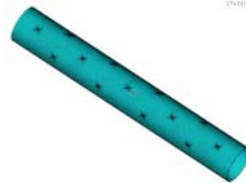
Fig.3 FEM model of piccolo structure
