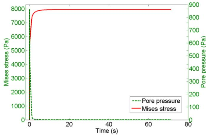
**Figure 8** The von Mises or solid skeleton stress and pore pressure versus time curves
