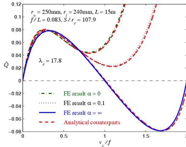
**Figure 6. Comparison between analytical and finite element results of limit point buckling of a crown-pinned CFST arch under a central concentrated load**
