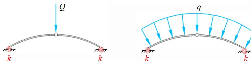
**Figure 1. Crown-pinned arches subjected to different loading cases**
