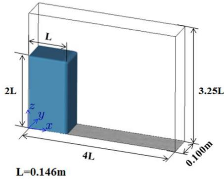
Figure 4. Computational domain and initial condition
