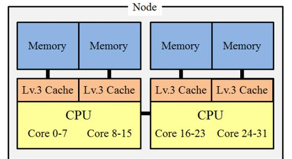
**Figure 2. Architecture of the CPUs and memories in a node**
