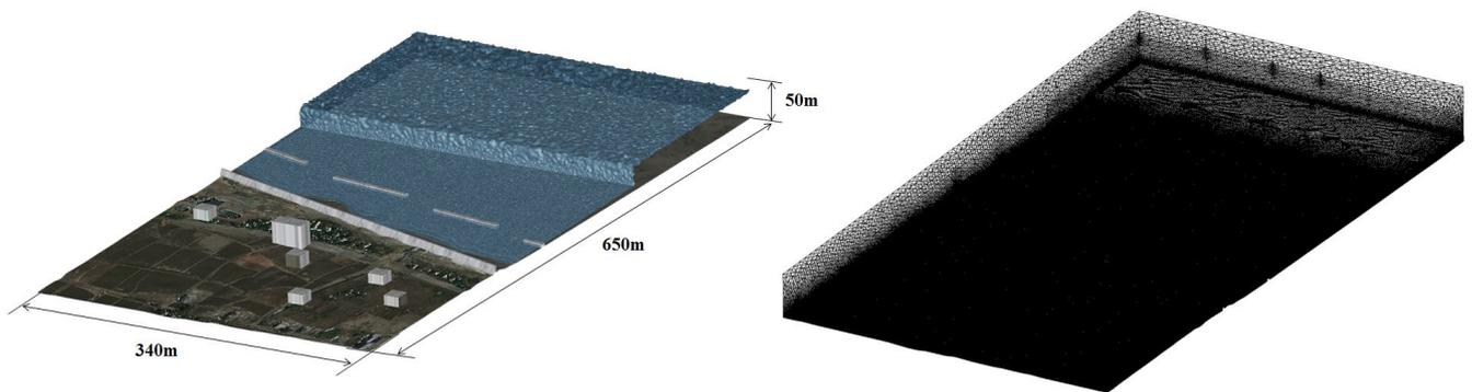
Figure 7. Initial condition and the finite element mesh
