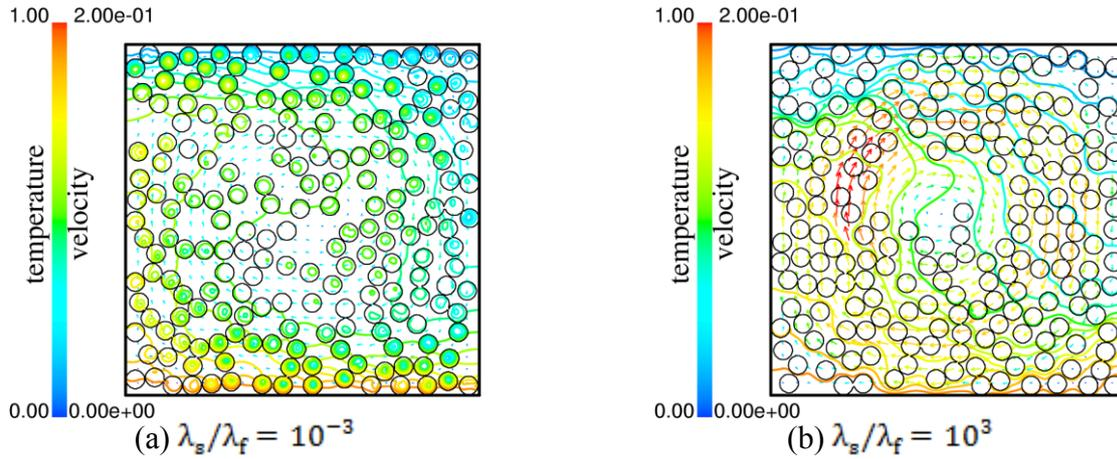
Figure 2: Instantaneous flow field and contours of temperature for different heat conductivities. Rayleigh number is  $10^5$  and bulk solid volume fraction is 38.5%. Colour shows the magnitude of the fluid velocity and iso-contour of temperature.
