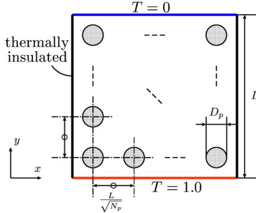
Figure 1: Schematic of arrangement of particles.
