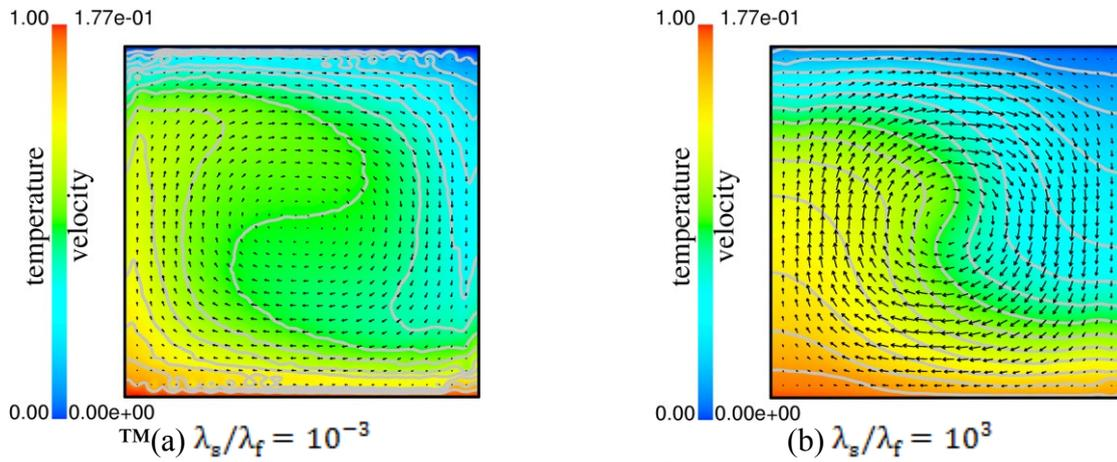
Figure 3: Time-averaged temperature and velocity fields for different heat conductivities. Rayleigh number is  $10^5$ . Average is taken between  $t = 500$  and  $1500$ . Magnitude the fluid velocity are levelled by colour, and iso-contours of temperature are plotted at constant intervals.
