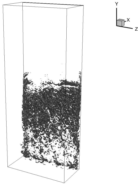
Figure 5. Coherent structures near the cold wall.
