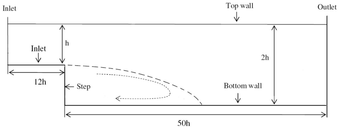
Fig. 1 Diagrammatic sketch of backward facing step
