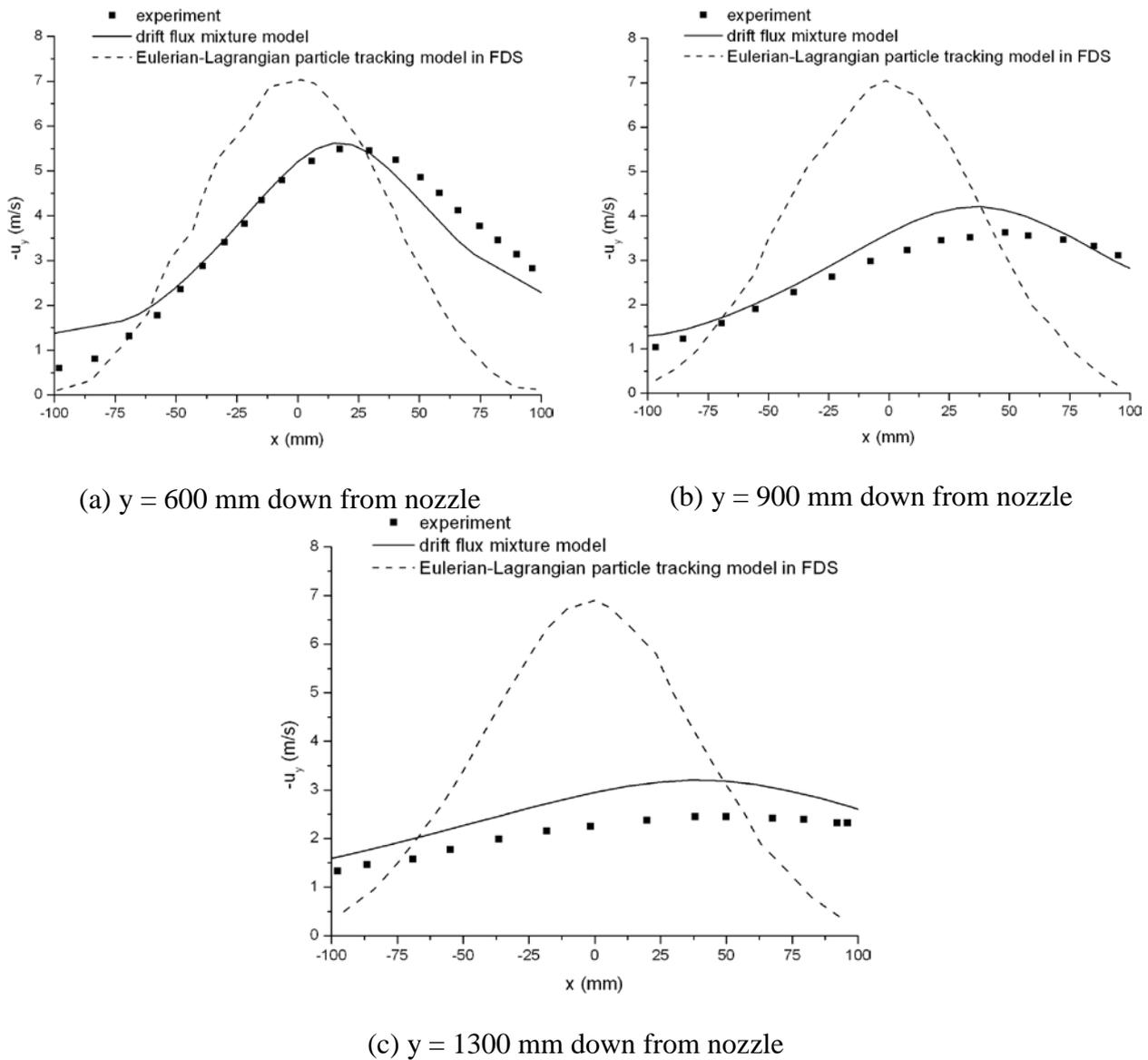
Fig. 7 Comparisons of water mist droplet velocity under different positions down from nozzle
