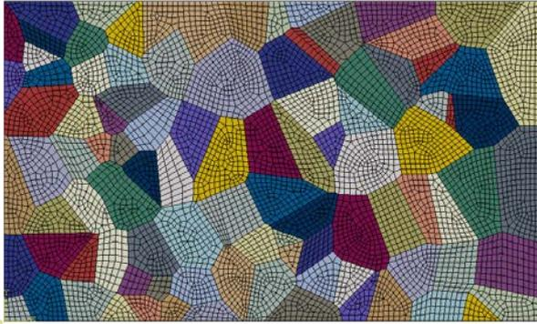
**Fig. 1. FE polycrystalline model (meshed)**
