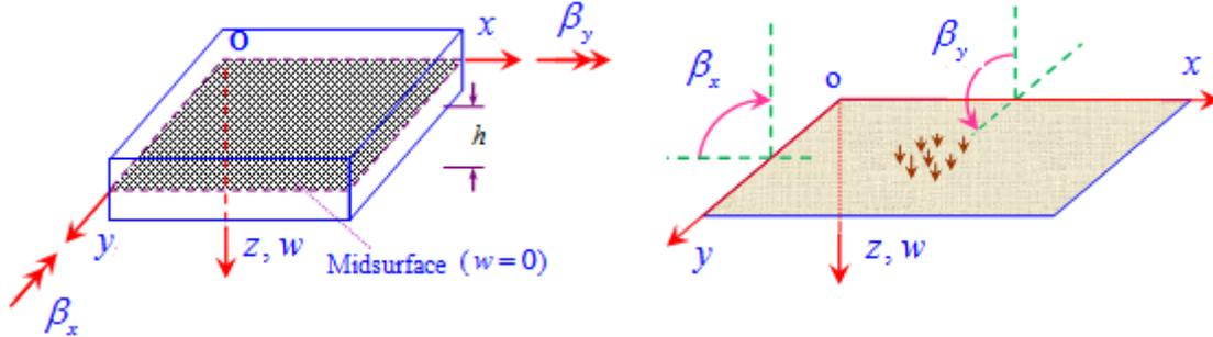
Figure 1. Mindlin plate and positive directions of deflection  $w$  and rotations  $\beta_x$ ,  $\beta_y$
