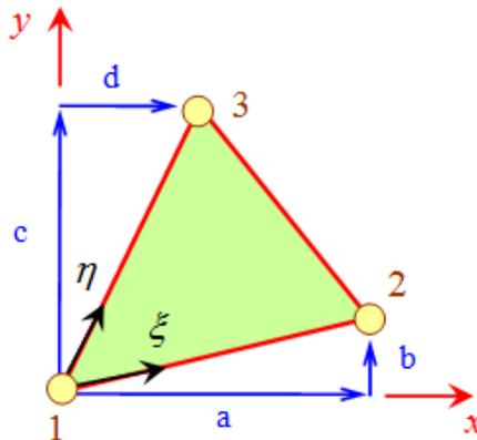
Figure 2. Three-node triangular element and local coordinates in the DSG3.
