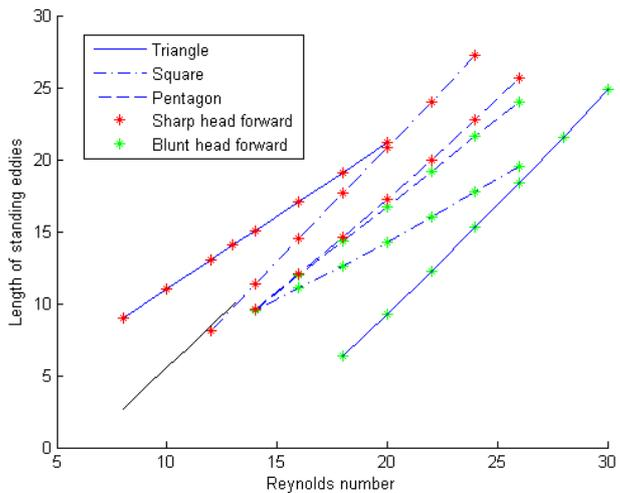
**Figure 2. Eddies' lengths of polygons. The black solid line represents circle cylinder**
