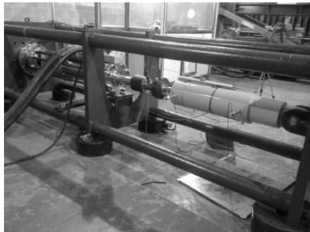
**Figure 1. View of the viscous test machine and fluid viscous damper**
