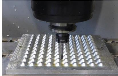
Figure 5: Milling cutter and work piece in Haas CNC milling machine
