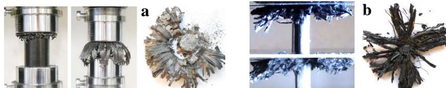
Figure 1 Failure modes of the composite tube and rods subject to crushing load (a. tube, b. rods)
