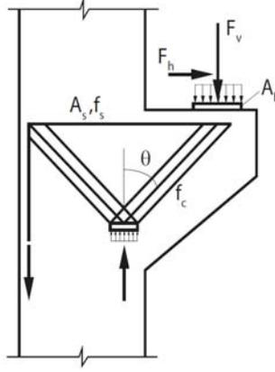
**Figure 1: Corbel Example. Strut-and-tie model.**
