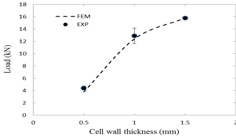
Figure 3. Comparison between measured and FE predictions for compression strength for CFRP as a function of cell wall thickness
