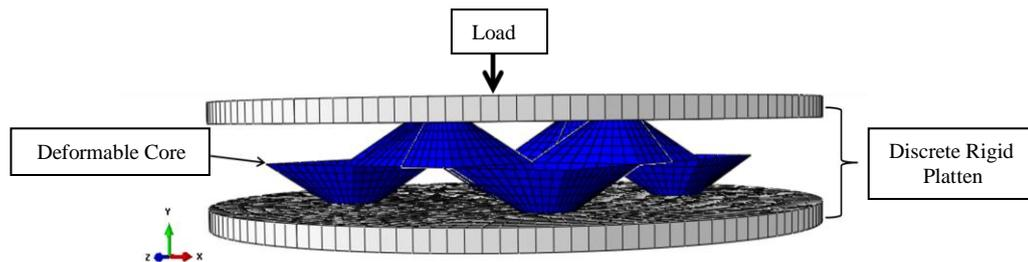
Figure 1. Loading conditions used in the contoured-core model
