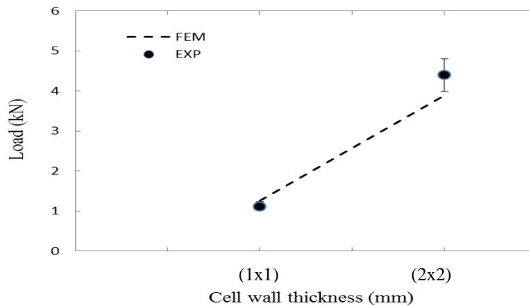
Figure 2. Comparison between measured and FE predictions for compression strength for CFRP as a function of number of unit cells
