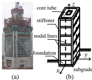
Figure 1: A mega-frame-core-tube system and its computational model
