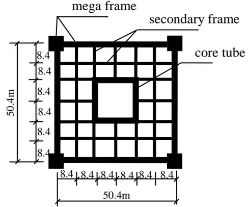
Figure 3. cross-section of a mega frame-core-tube system
