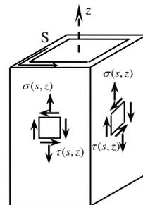
Figure 2: Stress state of the tube
