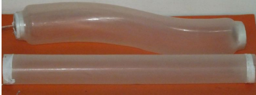
Figure 4. The air duct-shaped SMP mandrel with final deformable state and original state
