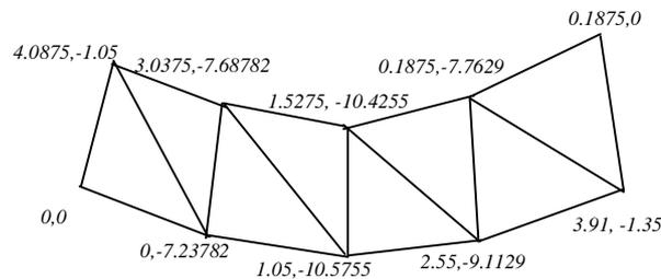
**Fig. 4. Classical Elastic deformed configuration of truss structure.**
