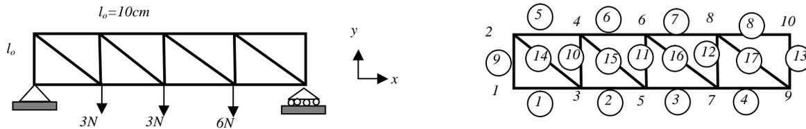
**Fig. 3. (a). Loaded Seventeen element truss structure (b) Numbering of nodes and elements.**
