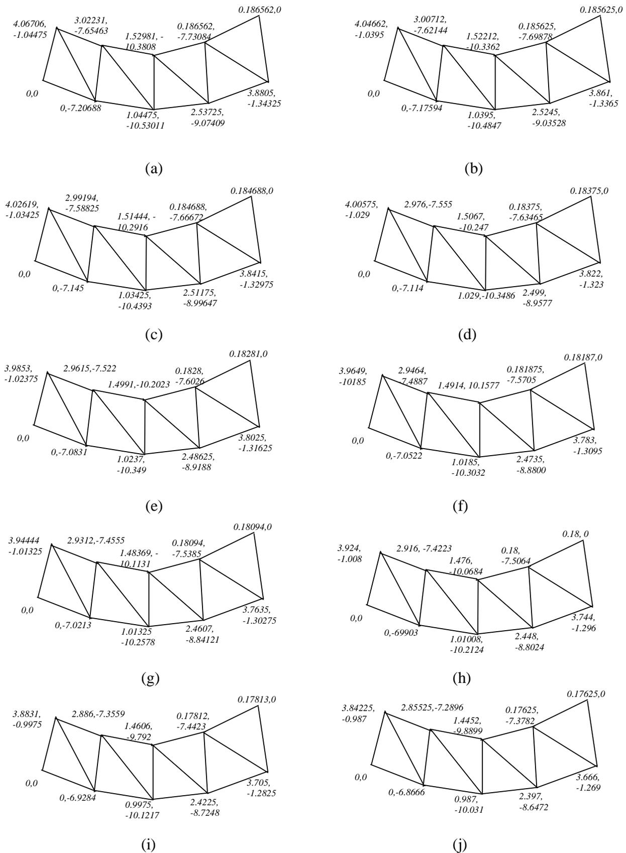
**Fig. 5. Gradient Elastic deformed configuration of structure. (a). ( $l_0 / \sqrt{c} = 20$ ); (b). ( $l_0 / \sqrt{c} = 10$ ); (c). ( $l_0 / \sqrt{c} = 6.7$ ); (d). ( $l_0 / \sqrt{c} = 5$ ); (e). ( $l_0 / \sqrt{c} = 4$ ); (f). ( $l_0 / \sqrt{c} = 3.3$ ); (g). ( $l_0 / \sqrt{c} = 2.85$ ); (h). ( $l_0 / \sqrt{c} = 2.5$ ); (i). ( $l_0 / \sqrt{c} = 2$ ); (j). ( $l_0 / \sqrt{c} = 1.7$ ).**
