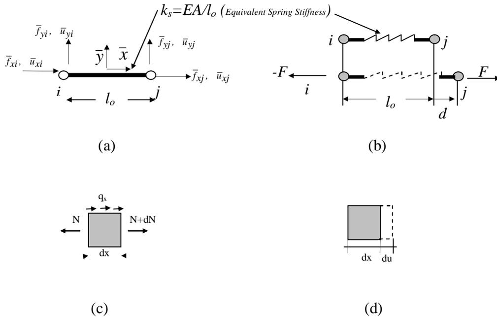
**Fig.1.(a). Generic 2-node truss bar element referred to its local coordinate system  $\{\bar{x}, \bar{y}\}$  with nodal forces  $f_{ij}$  and displacements  $u_{ij}$ . (b) Interpretation of a Generic truss element as equivalent spring (c) Equilibrium for infinitesimally small truss element. (d) Kinematics for infinitesimally small truss element.**
