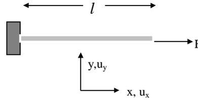
Fig.2. A bar under axial tensile load F
