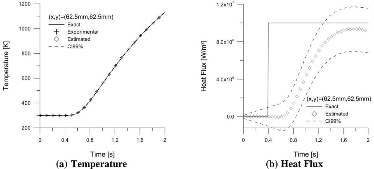
**Figure 4: Evolution of the reference and estimated values with time at  $(x, y) = (62.5; 62.5)\text{mm}$ .**
