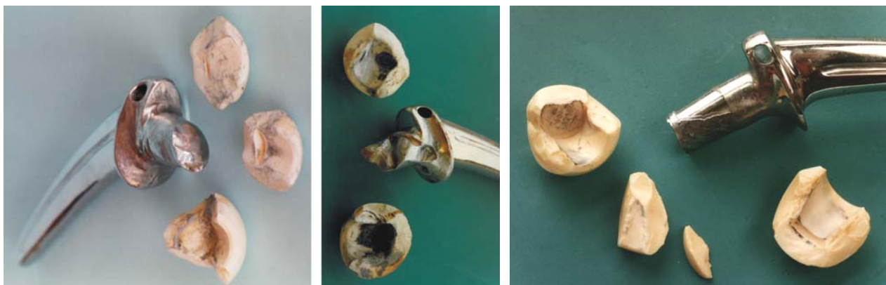
Figure 1. In vivo destroyed hip joint ceramic heads
