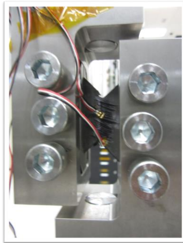
Figure 13: failure of carbon-epoxy specimen under shear loads
