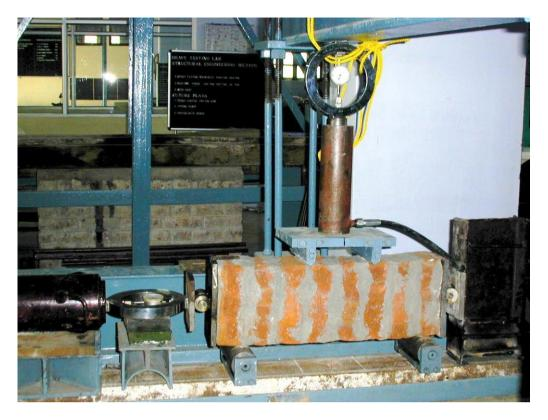
Figure 1b Test arrangements for determination of flexural bond strength of masonry
