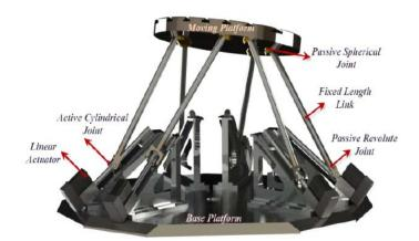
Figure 1. CAD model of 6-CRS parallel manipulator
