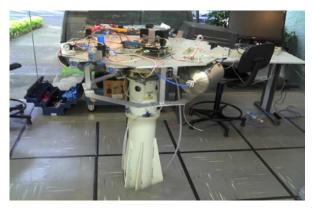
Figure 1- INPE 3-D simulator three reaction wheels.
