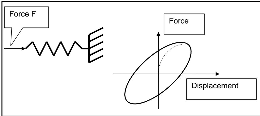
**Figure 1. Hysteresis of a spring-damper**
