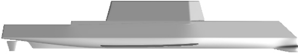
Figure 2 Geometry model of ONR Tumblehome (from Tokyo 2015 CFD Workshop)
