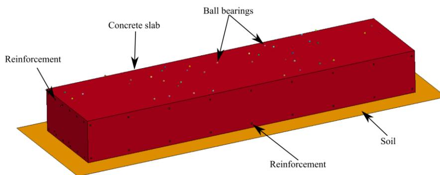
**Figure 1: FEA model including the ball bearing parts.**
