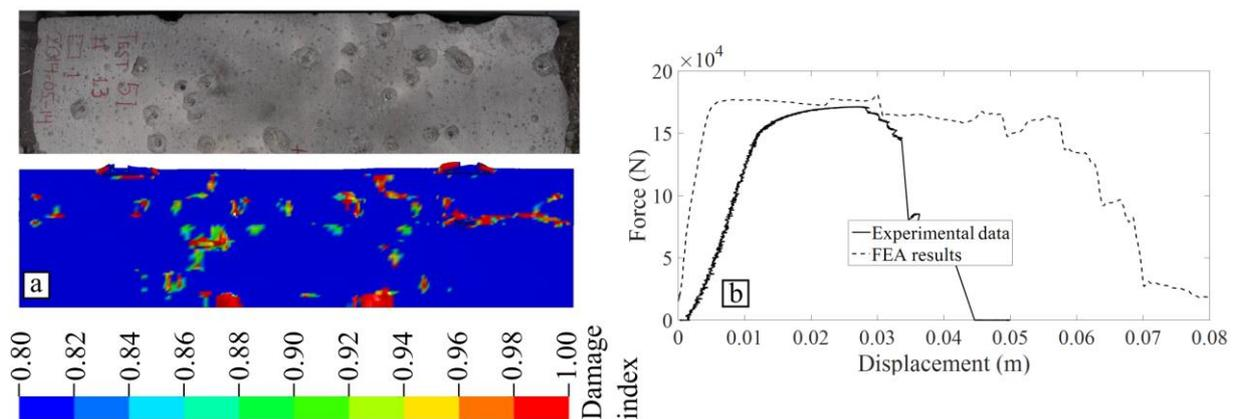
**Figure 2: (a) Dynamic damage on a typical slab. The FEA results show a similar damaged area to the experimental pictures. (b) Quasi-static force-displacement results.**
