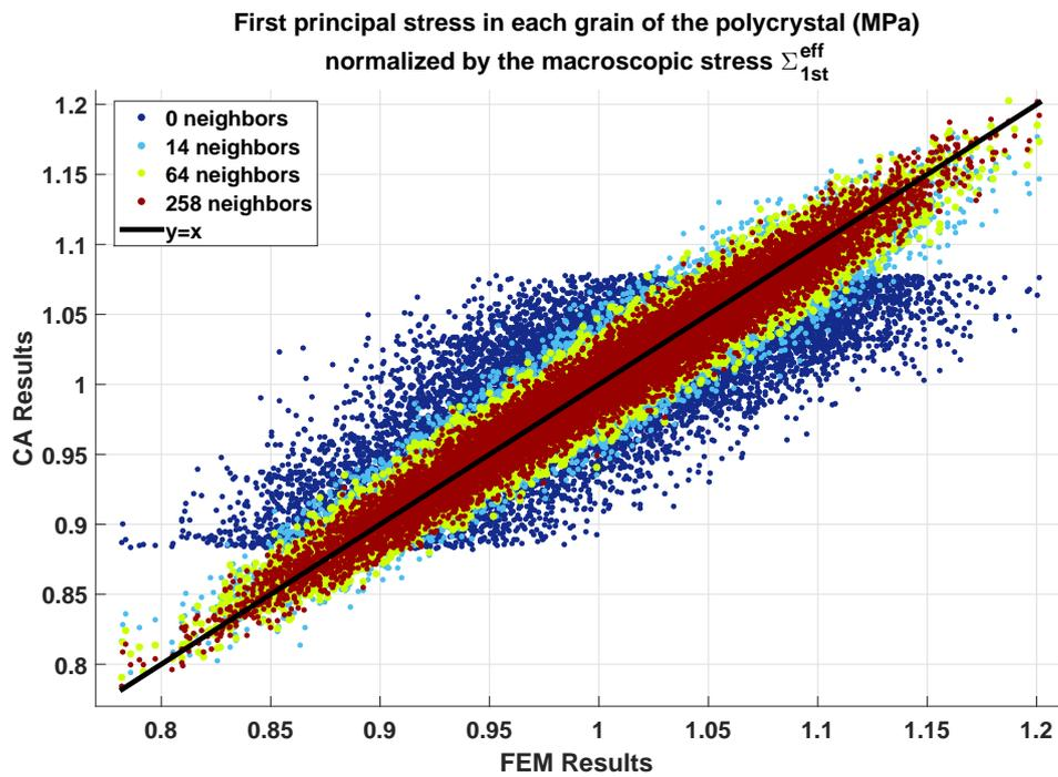
**Figure 8: Comparison of the FEM results with the CA results**
