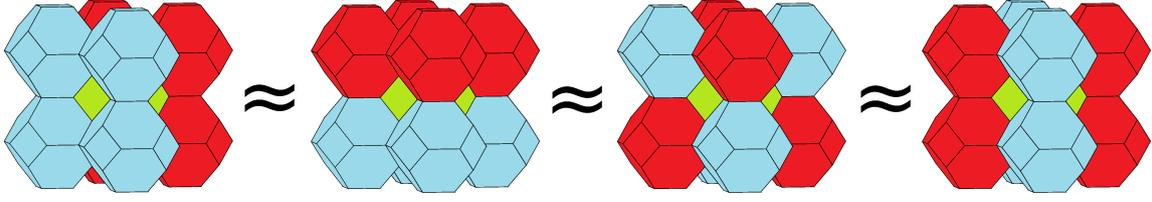
**Figure 6: Illustration of the influence of several grains with the same set of influence factors but with different repartitions (the grains in blue correspond to the lowest influence factor  $\alpha_{Bmin}^A$  and the grains in red to the highest influence factor  $\alpha_{Bmax}^A$ ): the influence of a neighboring grain on the central grain is not affected by the other neighboring grains.**
