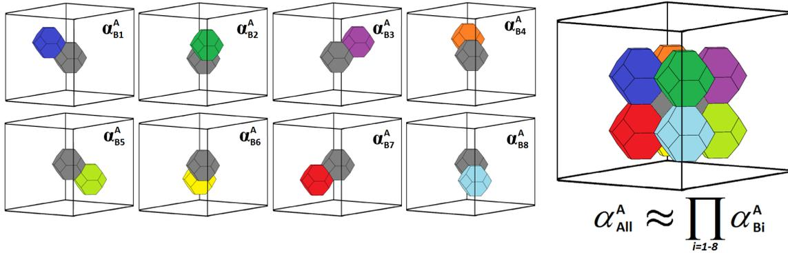
**Figure 5: Illustration of the influence of each individual grain compared to the influence of several grains (each color corresponds to a different crystallographic orientation): the influence of several grains is equal to the product of the influence factor of each neighboring grain**
