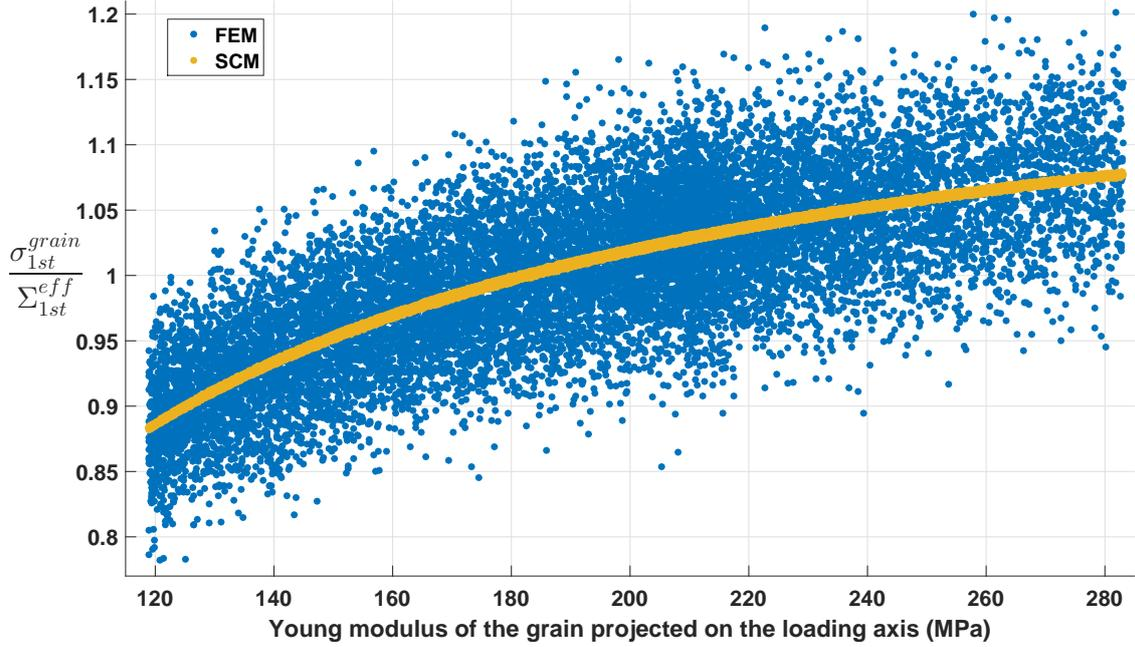
**Figure 2: First principal stress in each grain of the polycrystal normalized by the macroscopic first principal stress: Comparison between the FEM and the SCM**
