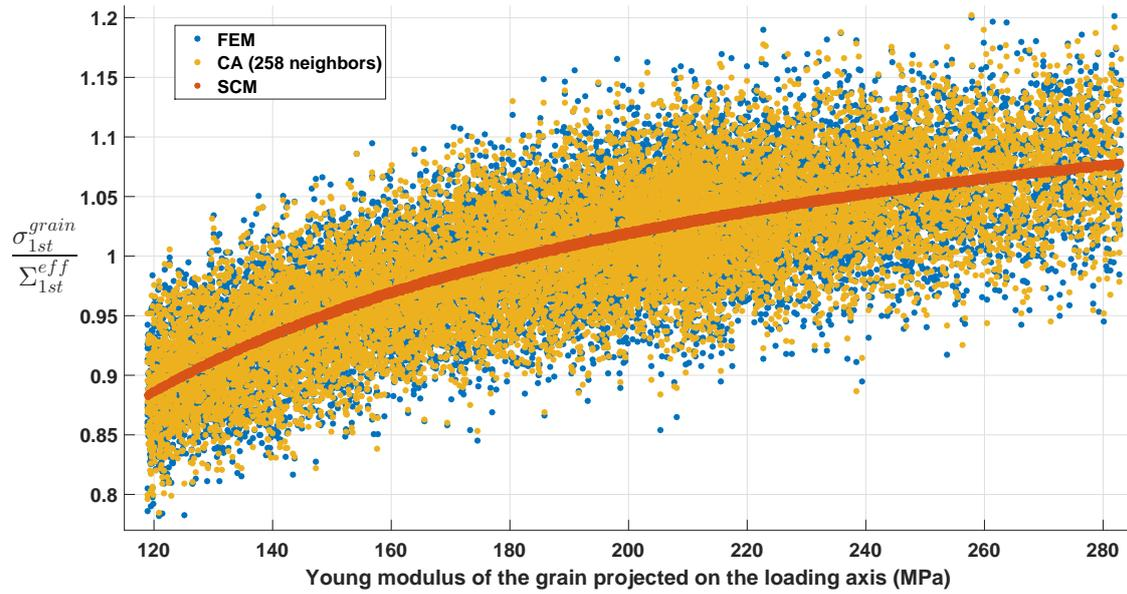
**Figure 7: First principal stress in each grain of the polycrystal normalized by the macroscopic first principal stress: Comparison between the FEM, SCM, and CA**
