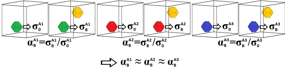
**Figure 4: Illustration of the first assumption (each color corresponds to a different crystallographic orientation): the influence of grain B on grain A is independent of the orientation of grain A**
