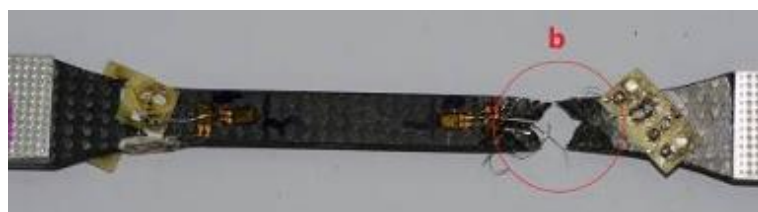
Fig 10 30°transverse tensile speicemen damage morphology
