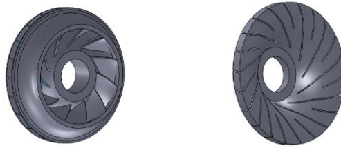
Figure 1. Impeller geometric model and flow channels model.
