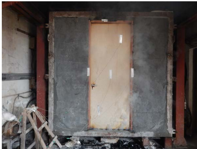
Figure 11. Unexposed surface condition of experiment at the time of 60 minutes
