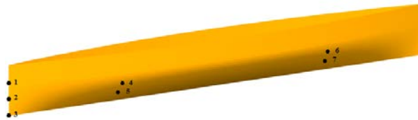
Figure 3. The control points distributed on Wigley hull by RBF method
