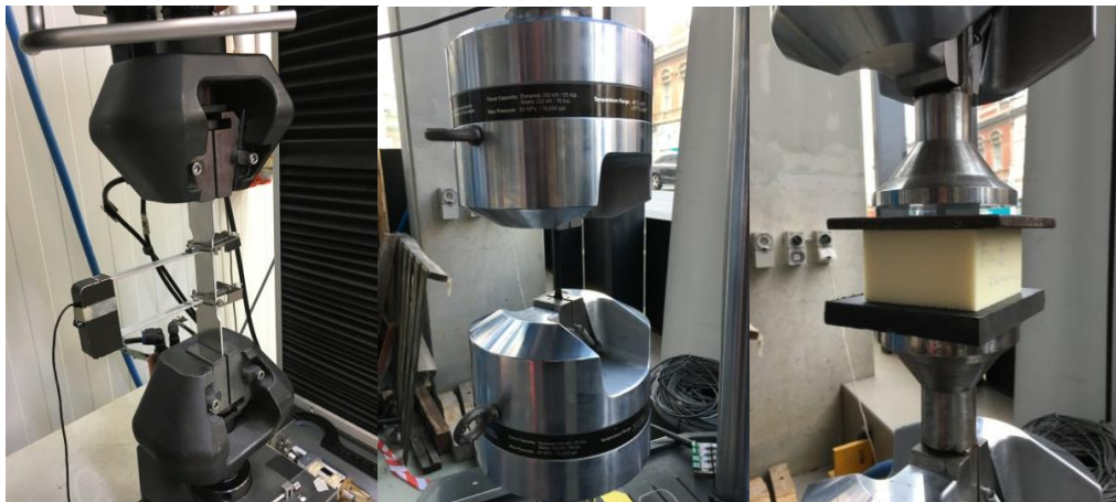
Figure 5 Left: Aluminium alloy tensile test; Middle: ABS plastic tensile test; Right: foam compression test
