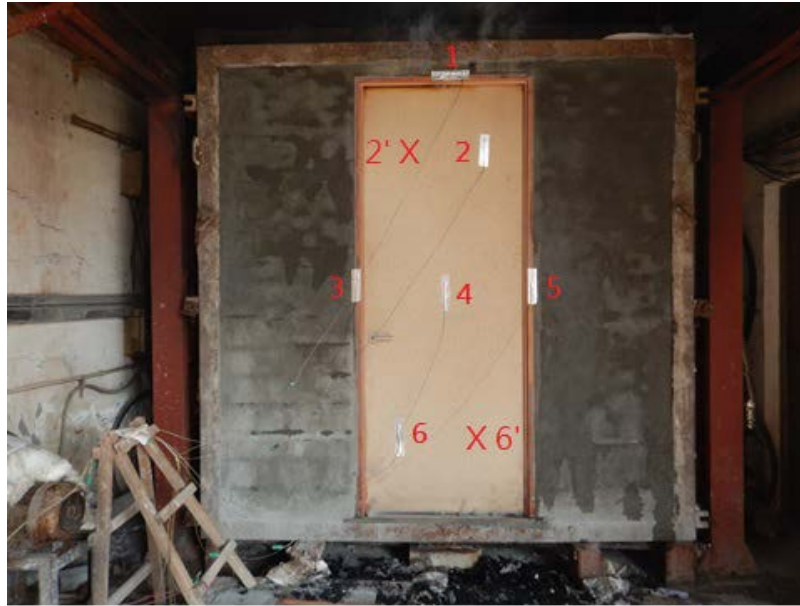
Figure 2. Single leaf - door installed on the furnace
