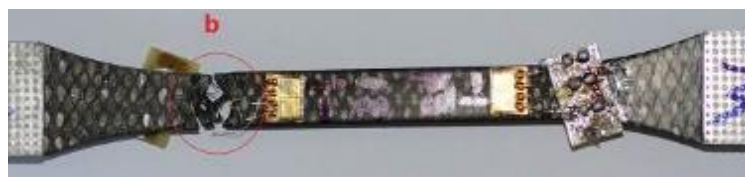
Fig 9 20° transverse tensile speicemen damage morphology
