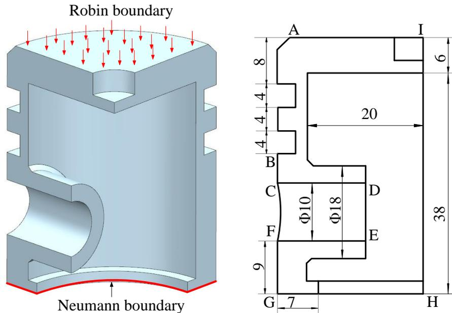
**Figure 5. The geometric parameters and the thermal boundary conditions of the piston model**
