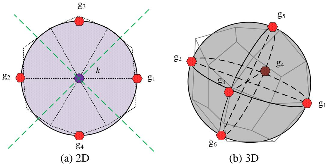
**Figure 2. The approximate integration domain and integration points for SNS-FEM**
