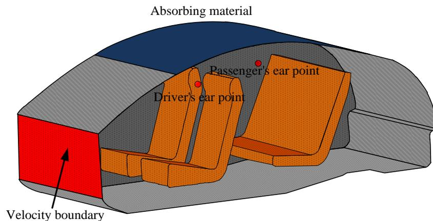
**Figure 3. 3D car passenger compartment with different kinds of boundary conditions**
