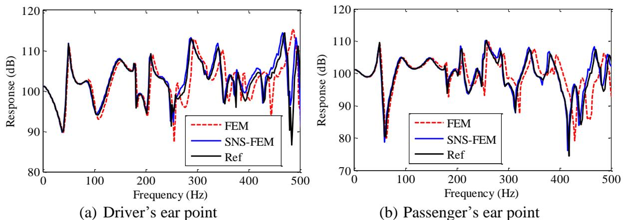
**Figure 4. The sound pressure levels at the driver's ear point and the passenger's ear point**
