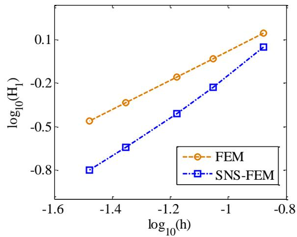
**Figure 9. Error estimation in  $H_1$  norm for 3D Poisson equation**
