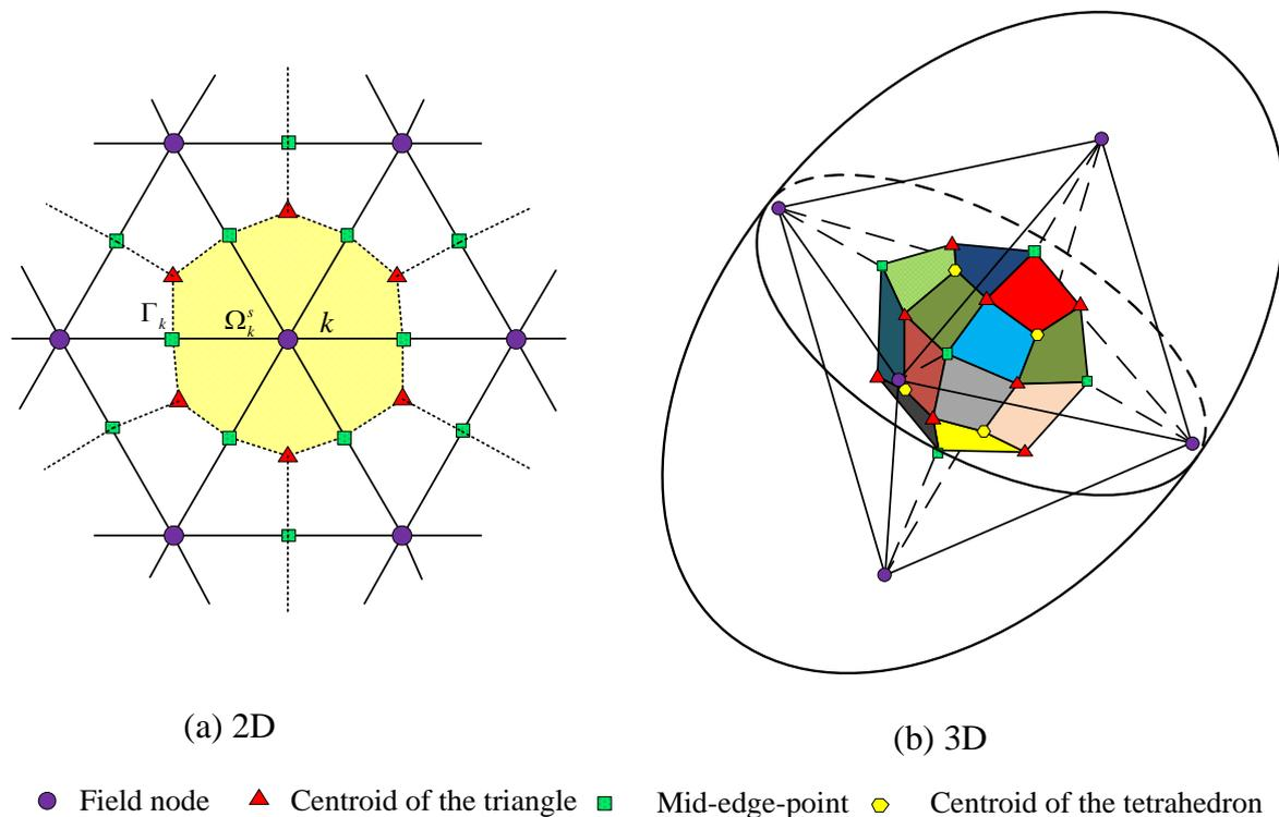
**Figure 1. A common process to construct the node-based smoothing domain**
