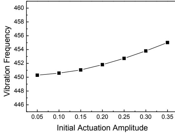
**Figure 5. The vibration frequencies vs initial actuation amplitude. In this situation, we apply different initial conditions' value on the spring-mass model. Then, the frequencies can be obtained from FFT analysis on the numerical results.**
