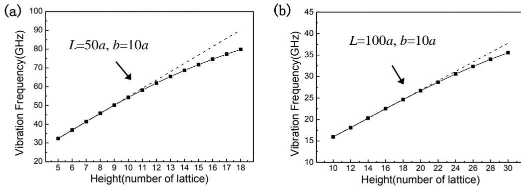
**Figure 6.** The solid lines in these figures represent the vibration frequencies in different heights. The dotted lines are the fitted straight lines based on vibration frequency values in the first five heights. In this situation, we use the frequencies obtained from FFT analysis on the MD simulations carried on different Fe nanowires. They are nanowires with the fixed  $L$  and  $b$  ((a)  $L=50a$ ,  $b=10a$ .(b)  $L=100a$ ,  $b=10a$ ).
