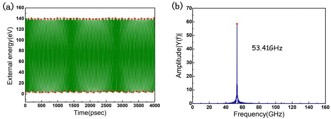
**Figure 3. (a) External energy time history of the Fe nanowire with the size of  $20a \times 10a \times 100a$  for a free vibration MD simulation at 0.2K. The simulation time is from 0 to 4000 picosecond. Circle markers highlight the maximum and minimum of external energy during each vibration circle. (b) The frequency spectrum from FFT analysis on the previous simulation (from 0 to 160 GHz). The star marker highlights the maximum of the main frequency component.**
