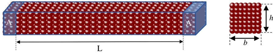
**Figure 1. A schematic visualization of a fixed-fixed Fe nanowire used in simulation. The atoms in the areas 'A' are fixed in all directions and the residual atoms can move freely.**
