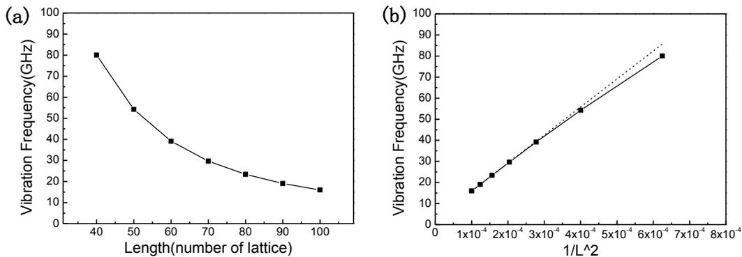
**Figure 7.** (a) The vibration frequencies vs nanowires' length. In this situation, we use the frequencies obtained from FFT analysis on the MD simulations carried on different Fe nanowires. They are nanowires with the fixed  $h=10a$  and  $b=10a$ . (b) The solid line shows the vibration frequencies vs  $1/L^2$ , while the dotted lines are the fitted straight lines based on vibration frequency values in the first three values of  $1/L^2$ .
