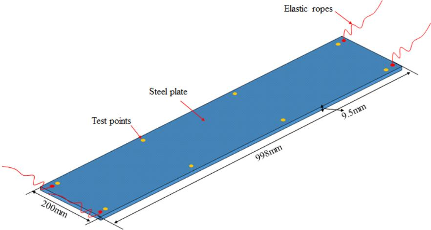
**Figure 2. The test modal and geometric parameter of the steel rectangle plate.**
