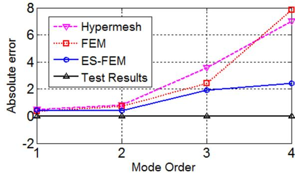
**Figure 4. Comparison on the error of nature frequency obtained from different methods**
