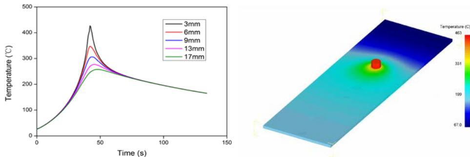
**Figure 1. Temperature histories and distribution in FSW**
