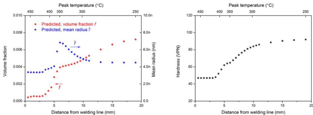
**Figure 3. Precipitations and mechanical properties in as-weld state**
