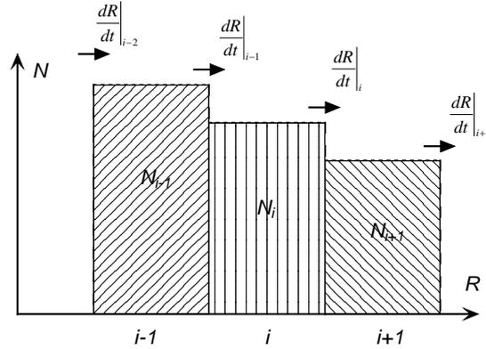
**Figure 2. Discretization in radius direction**
