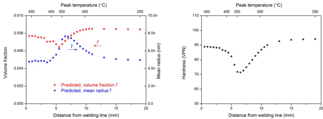
**Figure 4. Precipitations and mechanical properties after post-weld artificial aging at 180° C for 5 hrs**
