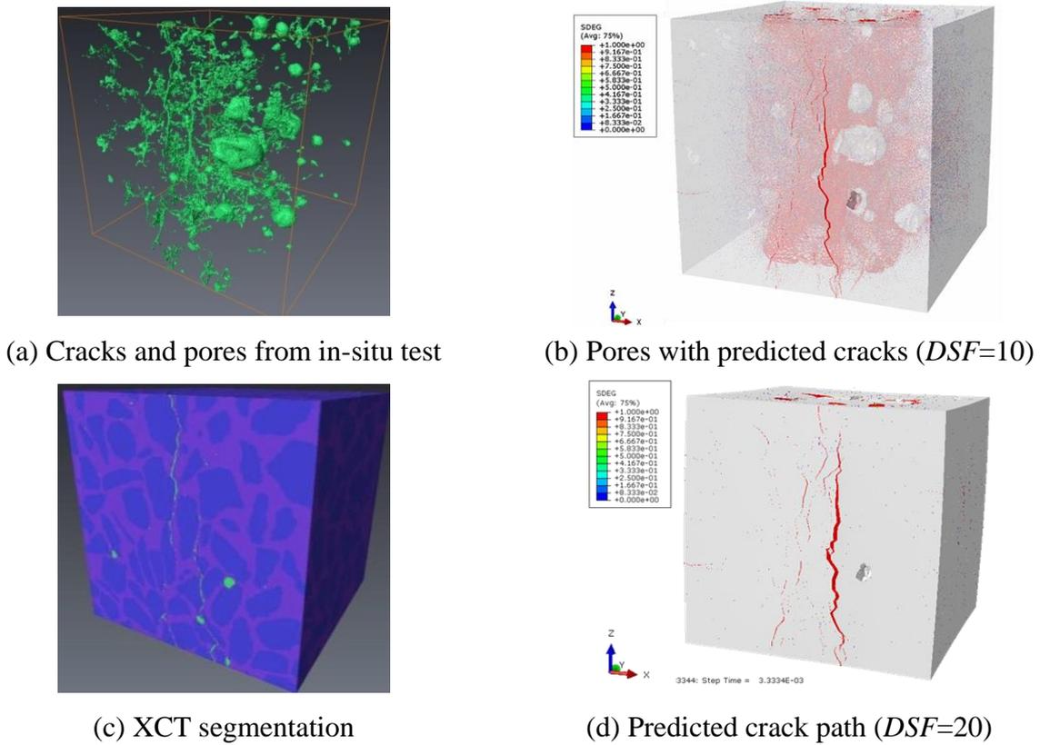
Figure 5. Comparison of cracks at peak load ( $DSF$ =deformation scale factor)
