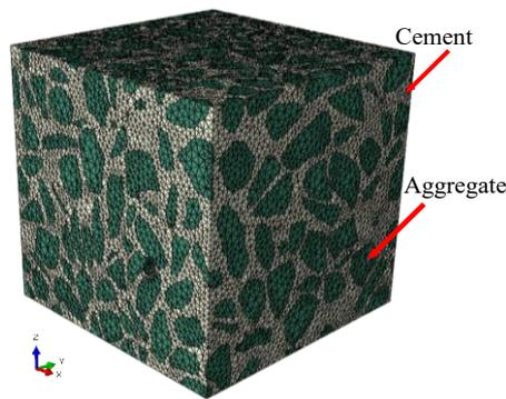
Figure 2. Generated 3D FE mesh
