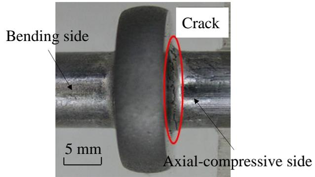
Fig. 3 Processed specimen exhibiting crack formation near the stepped section
