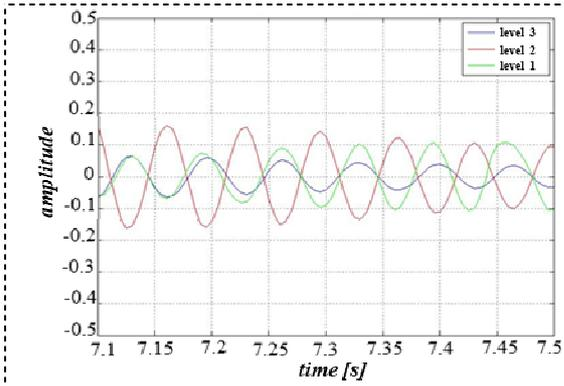
**Figure 10. Quasi-harmonic component with higher frequency (third component) of the dynamic response. PGA = 0,1g**
