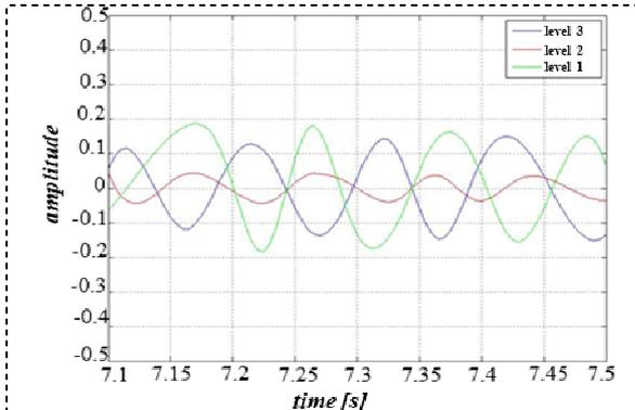
**Figure 8. Quasi-harmonic component with middle frequency (second component) of the dynamic response. PGA = 0,1g**
