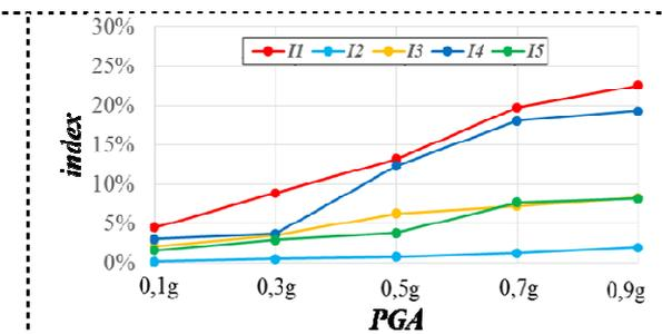
**Figure 19. Indices vs. PGA. Third mode shape**
