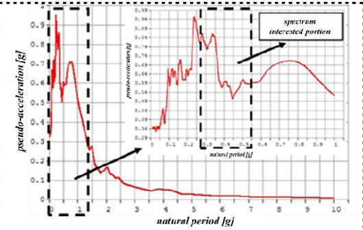
**Figure 3. Elastic response spectrum - Northridge earthquake, comp. 90°, 1994.**
