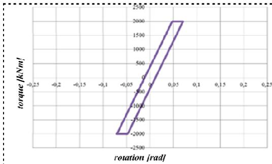
**Figure 12. Moment-rotation diagram of the plastic hinge at the column base (low damage)**
