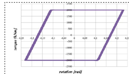
**Figure 14. Moment-rotation diagram of the plastic hinge at the column base (high damage)**
