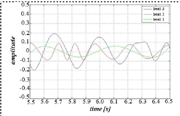
**Figure 6. Quasi-harmonic component with lower frequency (first component) of the dynamic response. PGA = 0,1g**
