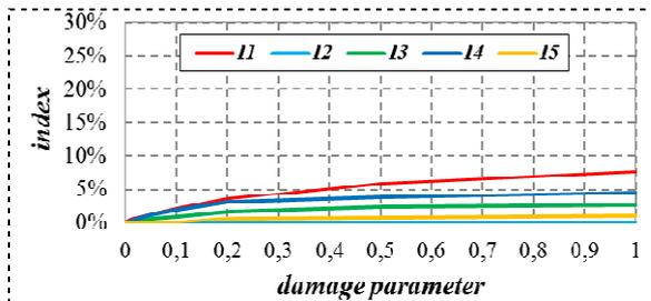
**Figure 16. Indices vs. damage parameter. First mode shape**
