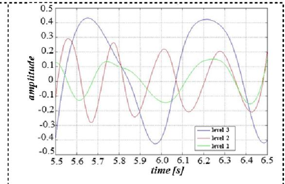
**Figure 7. Quasi-harmonic component with lower frequency (first component) of the dynamic response. PGA = 0,9g**
