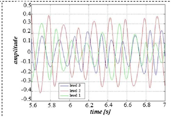
**Figure 11. Quasi-harmonic component with higher frequency (third component) of the dynamic response. PGA = 0,9g**
