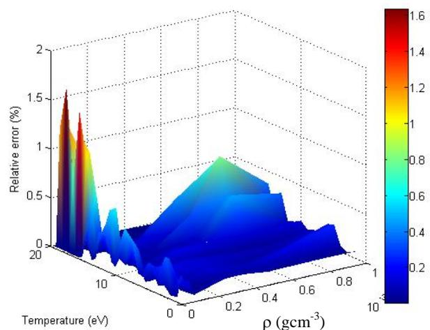
**Figure 2. Parametrization of the average ionization and radiative power loss for several mass densities and for the range of temperatures 1-20 eV for a Kr plasma. The figure also shows the relative errors in the fitting for values of the properties belonging or not to the database fitted.**
